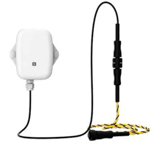
MPC6110-SN is a compact zone leakage detection sensor for detecting large area presence of water (or other liquids) and transmitting alarm using LoRaWAN® technology. With this low power consumption technology, MPC6110-SN can work up to 5 years with 4000 mAh battery. Combining with MobiCom Pro LoRaWAN® gateway and MobiCom Pro IoT Cloud solution, users can manage all sensor data remotely and visually and receive alarms via mobile APP.
